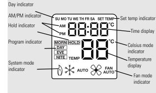
Figure 1: RAK163P1 and RAK147P1 Display
